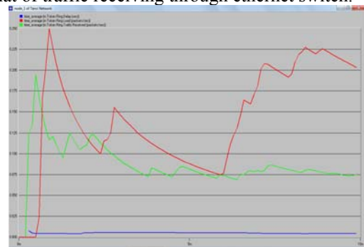
Figure 10:- Delay, Load and Traffic received through token ring of node_1 using TR4 network cable.
