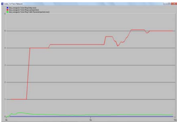
Figure 12:- Delay, Load and Traffic received through token ring of node_3 using TR4 network cable.
