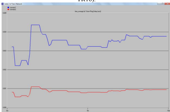
Figure 29:- Network Delay for node_5 for different types of cables (TR4 and TR16).
