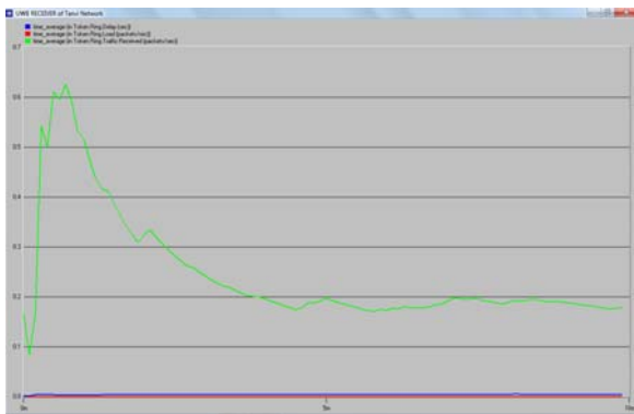
Figure 23:- Delay, Load and Traffic received through token ring of node_2
