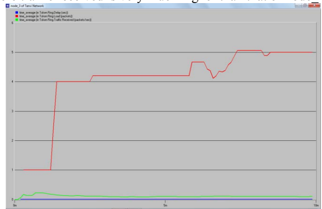
Figure 20:- Delay, Load and Traffic received through token ring of node_3 using Token Ring 16Mbps network cable.
